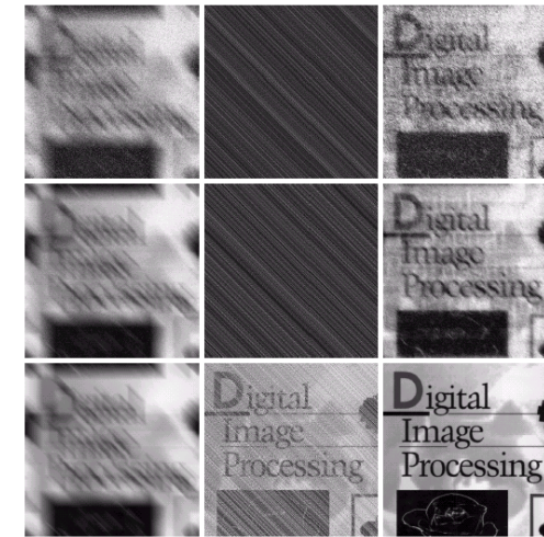
FIGURE 5.29 (a) Image corrupted by motion blur and additive noise. (b) Result of inverse filtering. (c) Result of Wiener filtering. (d)-(f) Same sequence, but with noise variance one order of magnitude less. (g)-(i) Same sequence, but noise variance reduced by five orders of magnitude from (a). Note in (h) how the deblurred image is quite visible through a "curtain" of noise.
