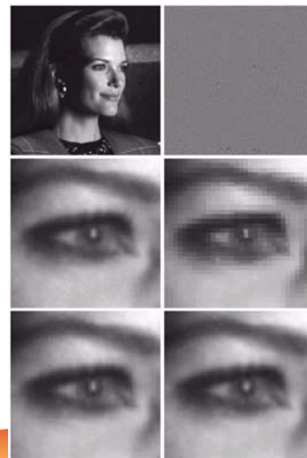
FIGURE 8.34 Approximations of Fig. 8.23 using 25% of the DCT coefficients: (a) and (b) 8 \times 8 subimage results; (c) zoomed original; (d) 2 \times 2 result; (e) 4 \times 4 result; and (f) 8 \times 8 result.
