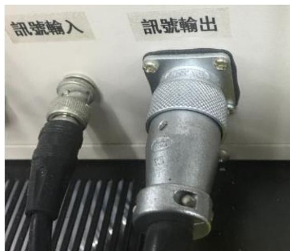
**2. Use BMC cable to connect Amplifier and Function generator, BCM cable connect the output signal of Function generator and the input signal of Amplifier.**
