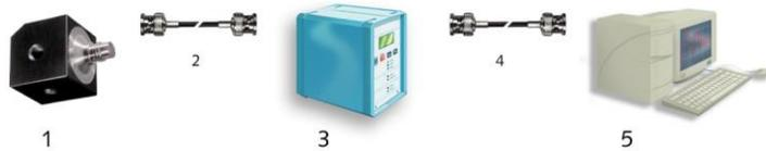
**Figure 2: Diagram of a Low Impedance Acceleration System**
