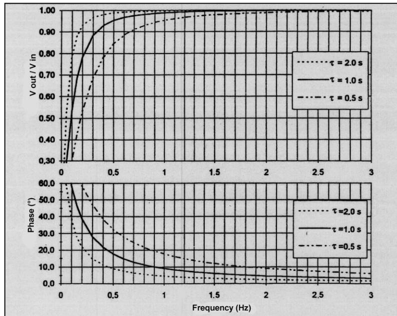
Figure 14: Frequency and Phase Response of Shock Accelerometers at Low Frequencies are Dependent on the Time Constant
