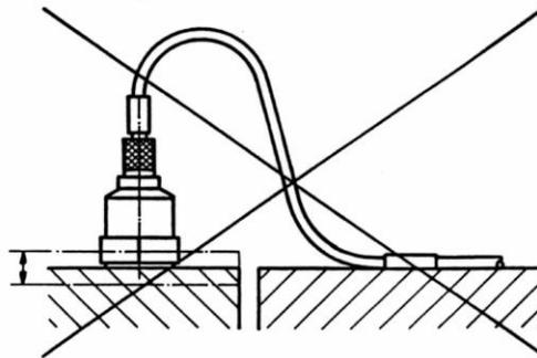
**Figure 5: Incorrect Cable Strain Relief**
