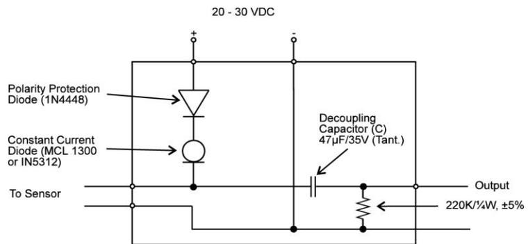
**Figure 7: Schematic Diagram Of A Simple Coupler**
