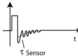
**Figure 11: Output Behavior During Overload and Recovery**
