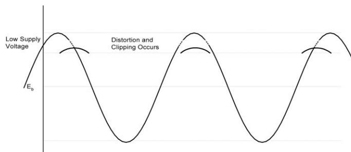
**Figure 9: Example of Output Distorting and Clipping when Supply Voltage is Low**
