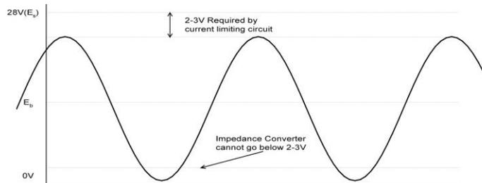
**Figure 8: Output Signal When Operated With 28V Supply**
