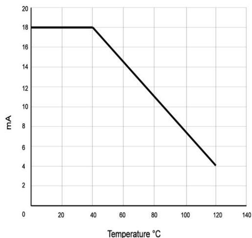
**Figure 12:** Maximum PIEZOTRON Current as a Function of Operating Temperature
