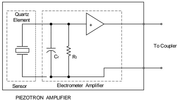
**Figure 6: Simplified Diagram of the Shock Accelerometer**
