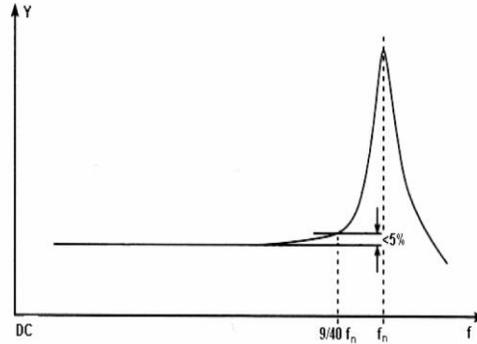
**Figure 13: Typical Frequency Response of a Piezoelectric Accelerometer**
